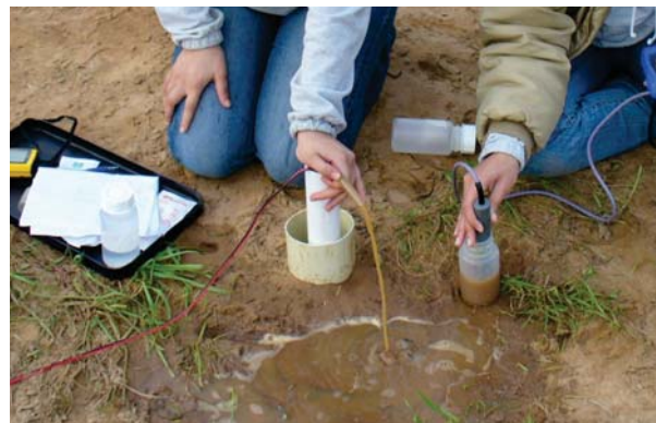
A plastic sampling bottle and handheld pH and electrical conductivity metres for field measurements.
