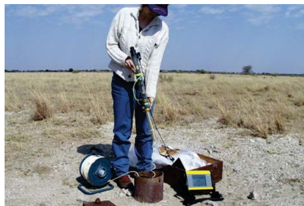
Examples of some of the types of electronic water level recording devices. Data is transferred directly to your laptop where evaluation of the data will take place.
