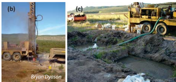
Air percussion drilling in the Karoo; b) Air percussion drilling in the West Coast region ; c) Mud rotary drilling.
