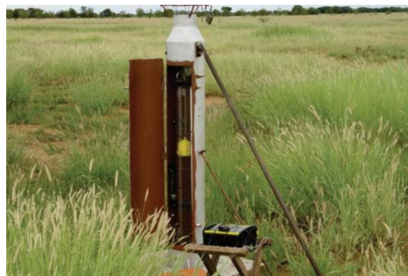
Rainfall gauges, developed by the DWS, used as part of the groundwater monitoring network in the country. The data can be stored electronically and then downloaded with a specific instrument.
