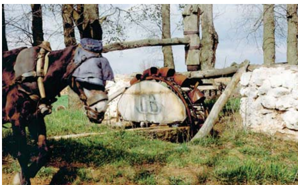
Some of the earliest methods of lifting water to the surface was with the use of a 'donkiepomp' or animal-driven pump.
