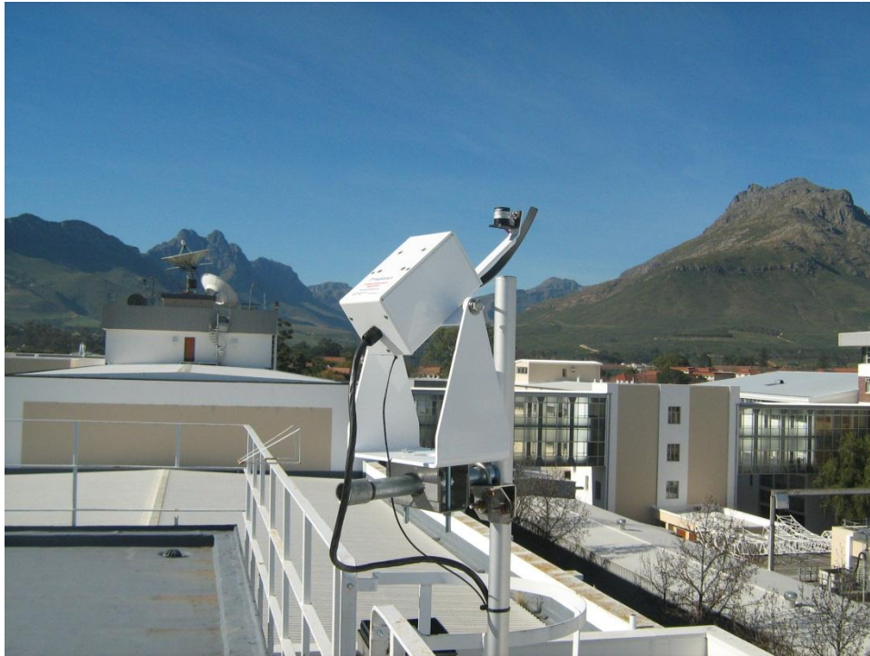
Fig. 4: An Irradiance RSR being tested at Stellenbosch University [11]
