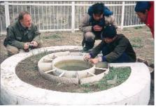
Installations of the water evaporation pan. (Left) A Canadian Class-A pan installed at the northernmost point on Earth where evaporation pans were used (79°25′N, 90°45′W). The pan is separated from the ground with a wood plank to avoid local effects from the ground. (Right) A Chinese pan at Hongwuyve, Tenshan Mountains. The pan is buried in an effort to minimize the effect of the exposed side wall.
